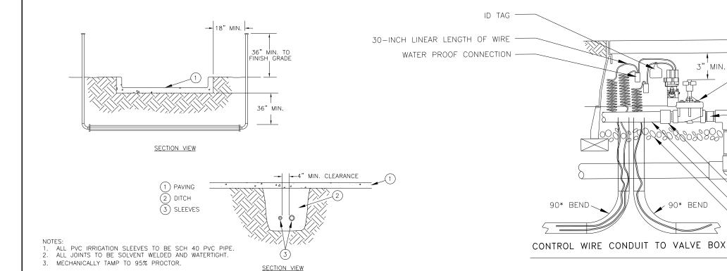
VALVE BOX WITH COVER: 12-INCH SIZE FINISH GRADE/TOP OF MULCH REMOTE CONTROL VALVE: IRRITROL MODEL 100P1 / 100P2
